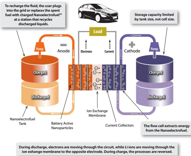
Taking advantage of Nanoelectrofuel’s unique properties, the flow cell design can be easily optimized by adjusting such variables as the size and composition of the nanoparticles and the size and shape of the flow cell materials. The Nanoelectrofuel can be stored externally to the flow cell and charged or discharged while passing through the cell in a closed circuit. Novel flow-through cells use inexpensive conductive materials.
